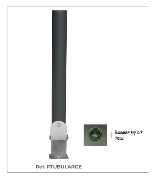
Removable tubular model bollard, built with iron tube with a diameter of ø 95 or 220 mm. and 2.5mm. of thickness. Total height of 1000 mm.
