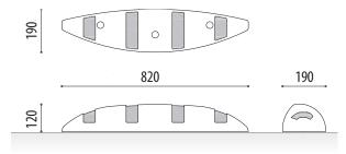
Pantera model road separator made with recycled material in 1 single piece measuring 820x190x120 mm. Black color and paint with white reflective microsphere.
