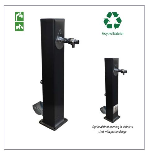
Fox urban plastic drinking fountains made of recycled thermoplastic polymer with independent push-button chrome-plated steel taps (people and animal use). Stainless steel drinker for animal use, with hole in the central part to avoid stagnant water and with side lever to tilt the drinker for later emptying.
